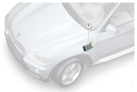
The AS control unit is integrated into the vehicle electrical system by the PT-CAN and the F-CAN. The AS control unit calculates the control signals for the AS actuating unit from various input signals.
